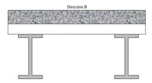
Our goal is to find an equivalent slab and beam system that can be modeled by finite elements analysis software. It is easily observed that the stiffness of the concrete filled deck will be different in both directions A and B, which is an orthotropic behavior. Some of the software can model orthotropic behavior in orthogonal directions such as ETABS and SAP2000, while other cannot such as GSA. We will consider both cases.
