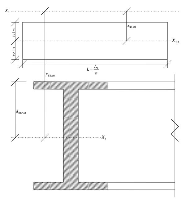
Herein,  $x_{\text{SLAB}}$  and  $x_{\text{BEAM}}$  are the offset distances of the shell and beam elements from the finite element surface, which is generally taken as the top of structural slab. Note that  $X_4$  is the beam neural axis.
